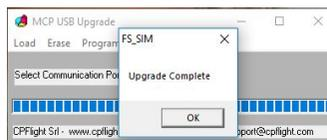
At the end it will appear a window that indicates the end of the programming. Close the upgrade program and disconnect the power supply from the MCP. Connect another time the power supply to verify that in the Right COURSE display window of your MCP will appear the new Firmware release number.
