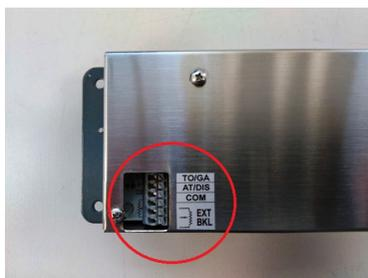
**WARNING!** The use of auxiliary connector is intended for expertise users. To use these auxiliary functions it is necessary to connect external switches/pushbuttons etc. Do not connect anything coming from any external power source or different by the following indications; warranty does not cover damages due to incorrect wiring of any external device.
